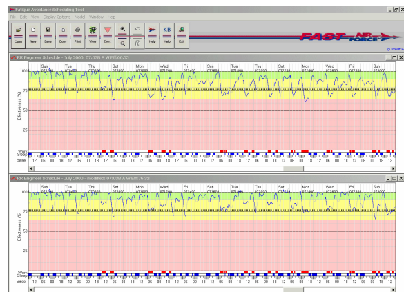
Figure 1: This is a screen image of the FAST main window and shows performance by a railroad engineer based on a log of sleep and on-duty time. The top window shows predicted performance based on actual sleep. The bottom window shows potential improved performance based on the addition of increased sleep during off-duty periods. The top of each graph shows the performance effectiveness at the day and time indicated by the vertical cursor.
